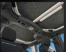
100% waterproof, headliner kit installs quickly without the need to remove your hard top. The individual pieces can be quickly installed by removing the specially designed tape and pressing firmly into place.
