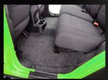
BedRug replaces vour OEM carpet. The 1/4-inch polypropylene foam backing with provided heat shields, insulates your interior from road noise.
