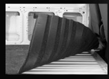
VanRug is die-cut and molded to fit each specific van application. Installs easily, and designed to fit under the edge of the cargo door step covers and rear plastic shroud for most applications.
