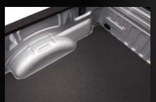
The TPO composite top layer construction offers a flat work surface, that is slip and skid resistant. The <sup>3</sup>/<sub>4</sub>" padded under layer provide dent and impact resistance while offering cushion for your knees.
